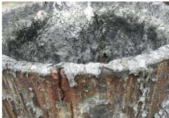
Figure 8. Crucible with 50 mm dross adhesion on inside surface after 42 days
