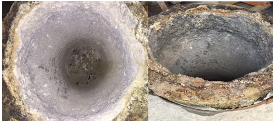
Figure 15. FUS 750 Z2 with PureCoat Coating with no dross adhesion
