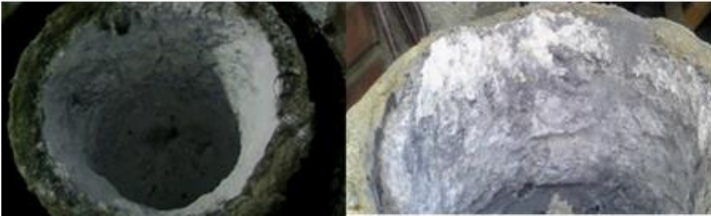
Figure 14. FUS 750 Z2 after using in Zinc distillation with a thick layer of dross
