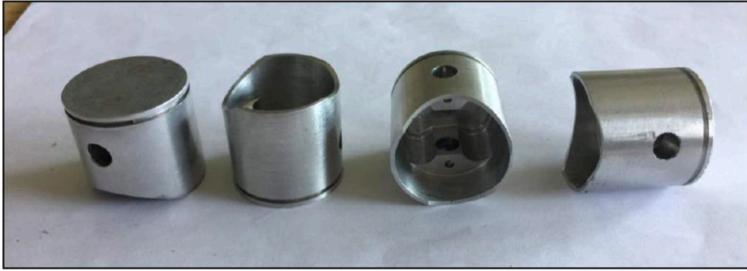
Figure 5 : Pistons after squeeze casting and machining
