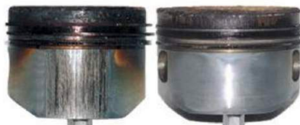
Figure 17 : The example of damaged pistons [16].
