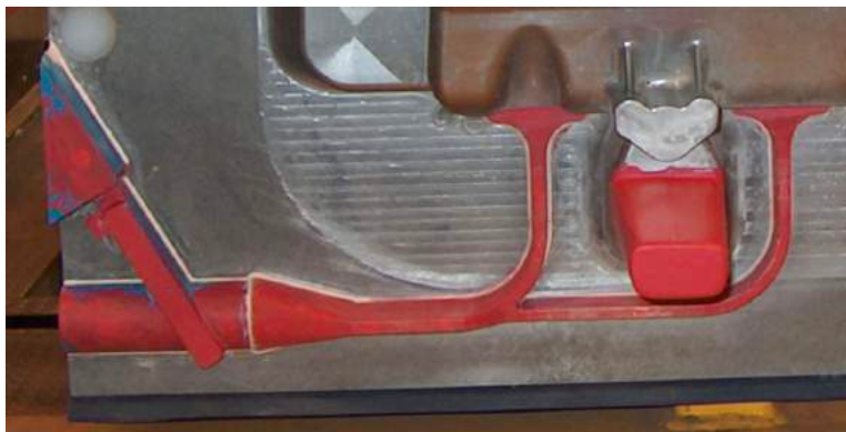
Figure 6 : Standard inlet pouring system on pattern plate
