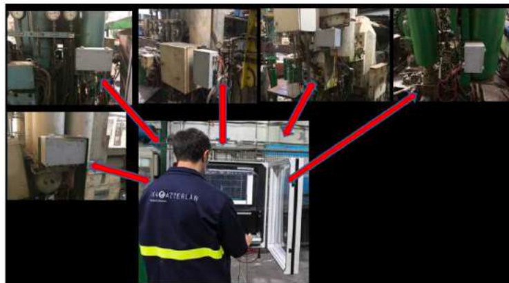
Figure 3 : Mobile HPDC specialized measuring system.
