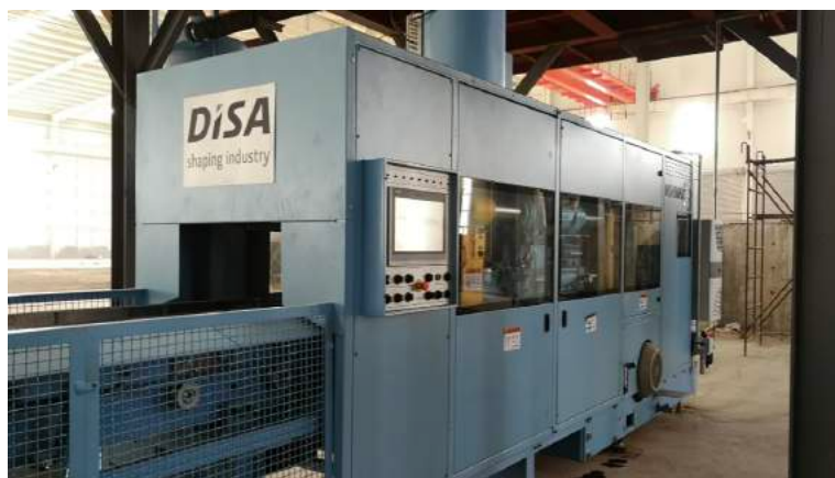
Figure 2: DISAMATIC C3-150-B with a mould size of 650x530 mm
