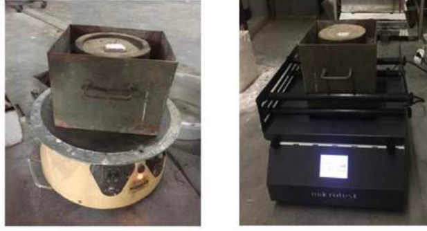
Figure 1: Vibration device used during moulding (left). Orbital shaking device used in the casting process of prepared moulds (right).
