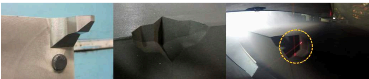
Figure 9 : Left (Reference blocks added to pattern plates) – Centre (Reference impressions the mould) – Right (Lasers measuring)
